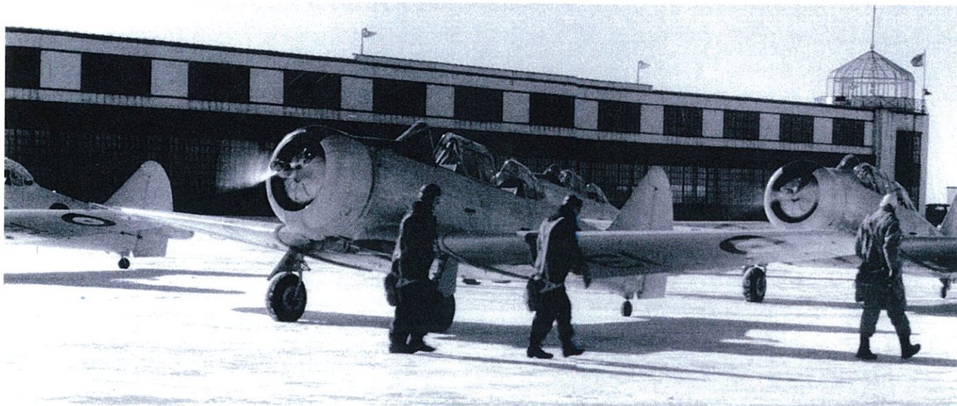
Harvard Is on the ramp at Trenton in 1940. No bush pilot hoping to fly in the RCAF would have a chance without first mastering the Harvard. Notice the careless practice of engines warming up with no one in the cockpit and no wheel chocks in place. (RCAF)
